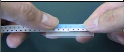
8 Rub the entire part of the Joint Tape with your finger to connect tapes completely.
