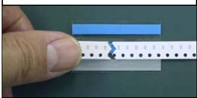
$\bigcirc$  Bend the Joint Tape along a bending line.
