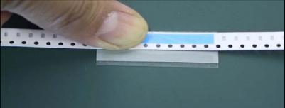
(9) Peel a transparent tape from the Joint Tape of a positioning guide.
