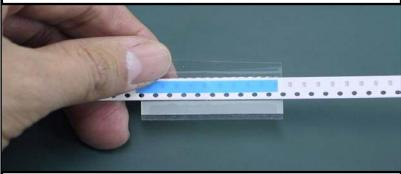
① All completed. ※Be sure a blue tape sticks completely to the carrier tape base.
